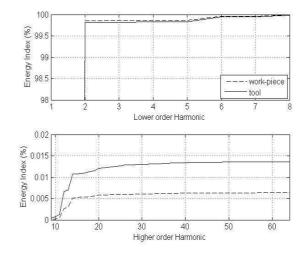
Figure 6: Energy Index for (a. 1-8 Harmonic Components and b. 8-64Harmonic Components).(NaNO<sub>3</sub>[-1 -1 0])
