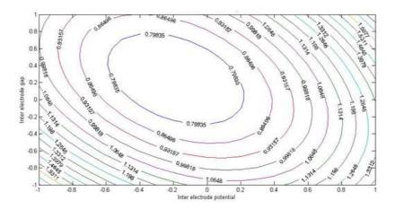
Figure 3: Variation of Overcut at Feed Rate = 0 (KCl+NaNO<sub>3</sub>\_1 Electrolyte)
