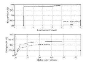
Figure 5: Energy Index for (a. 1-8 Harmonic Components and b. 8-64 Harmonic Components).(KCl[-1 0 1])
