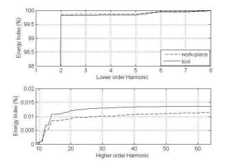
Figure 7: Energy Index for (a. 1-8 Harmonic Components and b. 8-64 Harmonic Components).(NaNO<sub>3</sub>+KCl [0 0 0])
