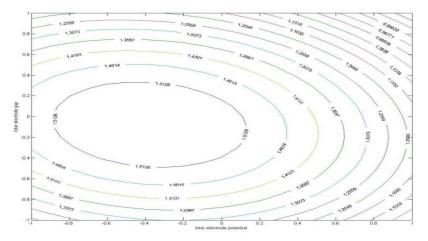
Figure 2: Variation of Overcut at Feed Rate = 0 (NaNO<sub>3</sub> Electrolyte)
